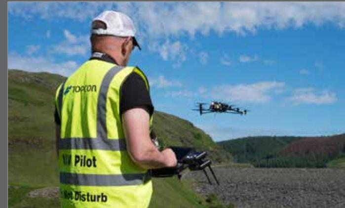
The Falcon 8 gives you full control over your flight planning. Manually fly the Falcon 8 around the object to be inspected, or program your flight path in advance. Save your accomplished flight path and repeat it automatically for exact comparison during a next inspection.
