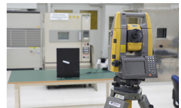
Auto-tracking durability test against rotating object.
